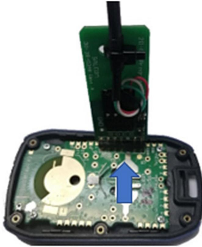
Figure 7: Programming Lead Position
