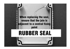
The middle two case screws may be sealed as an indicator to show that the unit has not been opened. If this is the case, remove the seal from these two screws. Remove the 6 stainless steel M3 slotted case screws and remove the back cover. Replace the battery with the designated type (see *Battery Type* below) ensuring the battery connector contacts are both tight.
