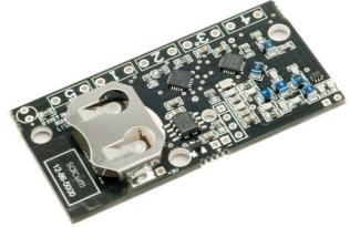
The **12-86-5005** transmitter PCB - upto 5 buttons, aerial & 1 LED fitted as options.
