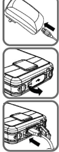
Plug the USB cable into the charger or to a computer USB port.
