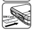
Insert SIM card into the SIM card slot with the Orientation shown. Push and release only when a "click" sound is heard.
