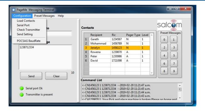
The package comprises the PageMe (Windows™) software application, a paging transmitter and a PC-to-transmitter interconnecting cable.
