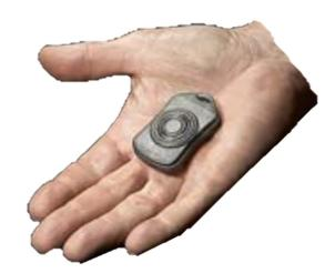
The 12-86 range of products are POCSAG direct to pager transmitters, allowing low cost systems to be developed since intermediate receivers and transmitters are not required for short range applications.
